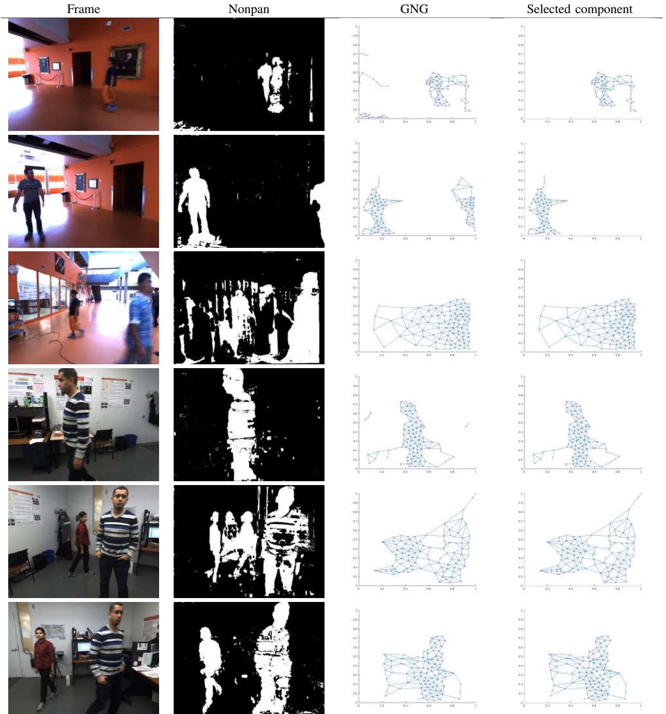
Figure 1. Graphical description of the operation of the proposed method. From left to right, the columns show a frame of a sequence, the binary mask produced by the nonpanoramic foreground detection method, the state of the neural network model in that moment (red circles to show the neurons and blue line segments to represent the connections among the neurons), the selected component (i.e. the largest connected component) and its centroid (represented with a green asterisk). The first and second rows show frame 78 of scenario3, each row with a different GNG initialization in the first frame.
