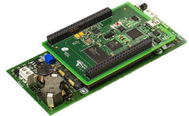
Fig. 2. SeaModem Power & DSP boards.
