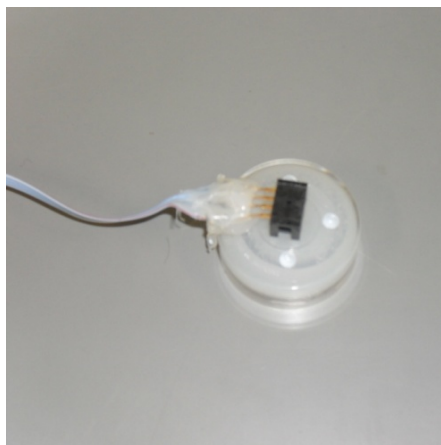
Figure 8: Pressure sensor Attached to Air Blocking Cap
