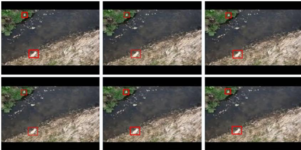
Figure 18. UAV-borne video capture (50 frames per seconds). Each panel shows water surface every 0.10 s. Red rectangles highlight the GCPs.
