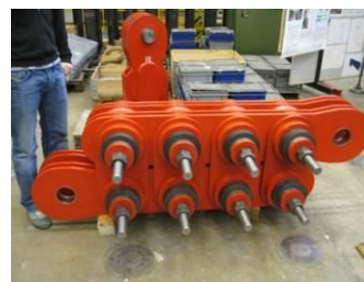
Figure 1B - Multi-joint large-capacity RFDs
