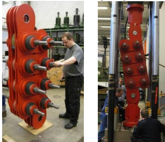
Figure 14 - 5000 kN Damper Tests at the Technical University of Denmark
