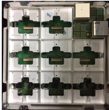
Figure 4: The mini X-ray detector of UBAT for ground test. There is an analog electronics, 2 YSO scintillation crystals and MAPMTs set on right-upper side of the UBAT detector structure.
