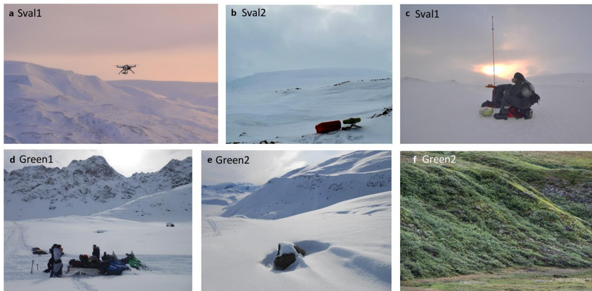
Figure 2. (a) The minimal set-up during the image acquisition phase for area Sval1 in overcast/fair conditions. (b) Global Navigation Satellite System (GNSS) data acquisition phase using the JAVAD antenna and receiver for area Sval2. Overcast and sastrugi sculpted snow can be observed. (c) Snow depth probing on a GCP location for area Sval1 during overcast conditions. (d) Survey preparation for area Green1 during fair conditions on completely fresh and featureless smooth snow. (e) Featureless conditions of area Green2 in clear/fair sky. (f) Typical low vegetation shrubs (5 to 30 cm) found in Arctic regions.
