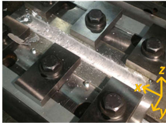
Figure 2. Photo of the welding setup including the clamping system and a finalized welding scar from the 20 mm rotating tool.
