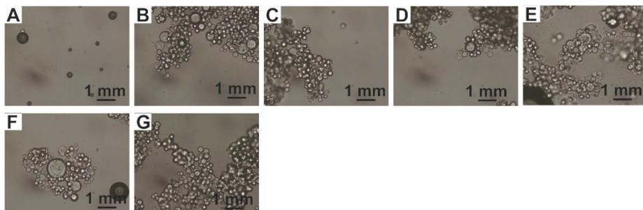
**Figure S3** Optical microscopy images of surface functionalized OSTE-1000 particles via TEC using different allyl and vinyl monomers, A) OSTE-AMA, B) OSTE-AA, C) OSTE-Vim, D) OSTE-Aam, E) OSTE.APFB, F) OSTE-ATFA, G) OSTE-AGE
