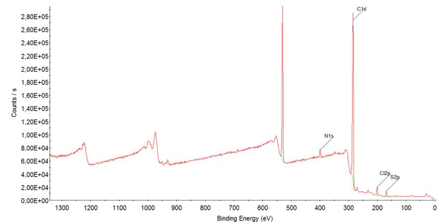
**Figure S7** XPS spectrum of PSf membrane surface grafted by CuAAC with alkyne-pPEGMA (PSf-5)
