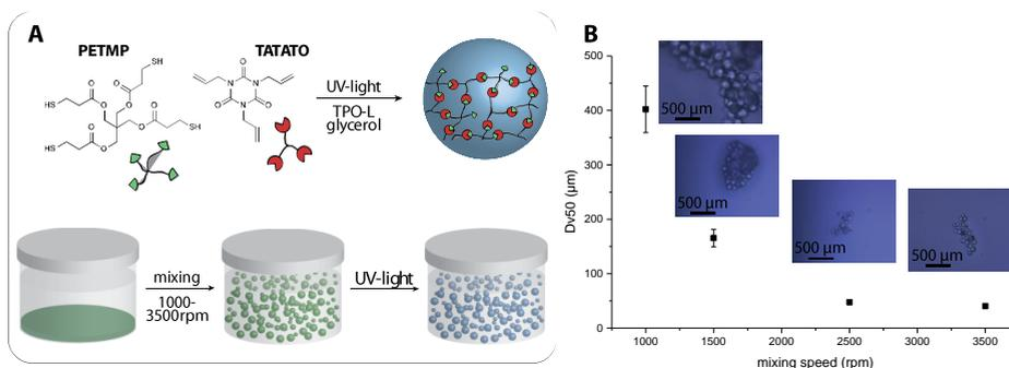
**Figure 4-2** A) Preparation of OSTE microparticles via suspension in a speedmixer followed by subsequent photochemical cross-linking of PETMP and TATATO. B) Particle size (Dv50) as a function of mixing speed with optical microscopy images (50 x magnification) of the OSTE particles.
