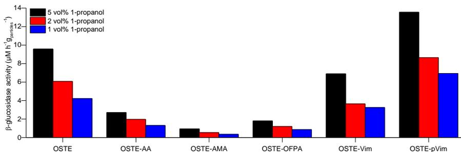
**Figure 1.** Activity (combined initial reaction rates of trans-glycosylation and hydrolysis) of  $\beta$ -glucosidase immobilized on pristine (OSTE) and functional OSTE particles OSTE-AA, OSTE-AMA, OSTE-OFPA, OSTE-Vim and OSTE-pVim in solutions with different 1-propanol contents, such as 5, 2 and 1 vol%
