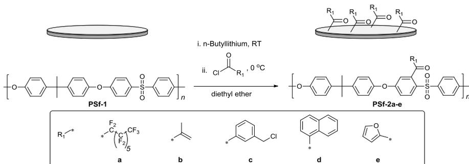
**Scheme 7-1** PSf membranes (PSf-1) were lithiated with n-butyl lithium (n-BuLi), and subsequently acylated using pentadecafluorooctanoyl chloride (a), methacryloyl chloride (b), 3-(chloromethyl)benzoyl chloride (c), 1-naphthoyl chloride (d) and 2-furoyl chloride (e) in order to obtain small molecular weight functional PSf membranes PSf-2a-e.
