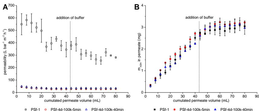
**Figure 7-4** Comparison between permeability (A) and amount of enzyme collected in the permeate during ADH (B) immobilization on pristine PSf membrane (PSf-1) and pVim grafted PSf membranes for 5 and 40 min (PSf-4d-100k-5min and PSf-4d-100k-40min)
