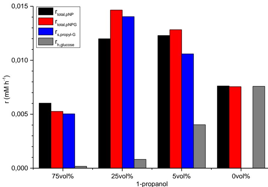
**Figure S1.** Overall initial reaction rates for the conversion of pNPG ( $r_{\text{total,pNPG}}$ ) and the formation of pNP ( $r_{\text{total,pNP}}$ ), as well as for the individual trans-glycosylation ( $r_{\text{s,propyl-G}}$ ) and hydrolysis ( $r_{\text{h,glucose}}$ ) reactions between pNPG, water and 1-propanol by  $\beta$ -glucosidase from *Thermotoga neapolitana* in solution
