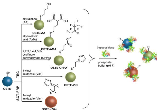
**Scheme 5-1** Surface functionalization of OSTE particles via thiol-ene chemistry (TEC) using Vim, AA, AMA, and OFPA introducing a functional monolayer; and via surface chain transfer free radical polymerization (SCT-FRP) using Vim grafting the surface with a dense polymer layer (pVim) followed by immobilization of  $\beta$ -glucosidase on pristine and functional OSTE particles
