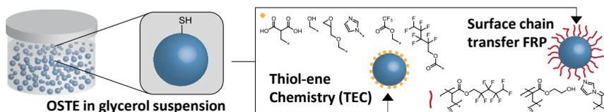
**Figure 4-1** Illustration of prepared OSTE particles, which were subsequently surface functionalized by means of TEC and surface chain transfer free radical polymerization (SCT-FRP)
