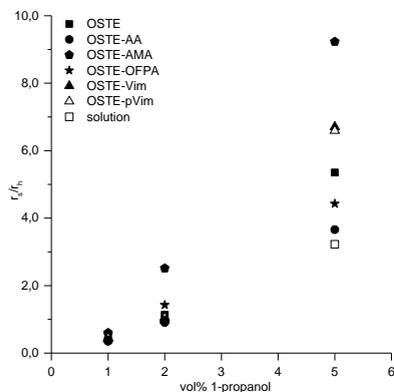
**Figure 3.** Selectivity ( $r_s/r_h$ ) between trans-glycosylation (s) and hydrolysis (h) of pNPG catalyzed by  $\beta$ -glucosidase immobilized on pristine (OSTE) and functionalized OSTE particles OSTE-AA, OSTE-AMA, OSTE-OFPA, OSTE-Vim and OSTE-pVim at different 1-propanol contents
