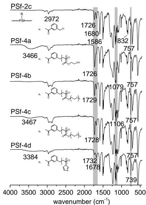
**Figure S2** IR spectra of polymer grafted PSf membranes post functionalization, top: via SI-ATRP including activated 3-(chloromethyl)benzoyl PSf membrane, grafted with polyHEMA (PSf-4a), polyMPEGMA (PSf-4b), polyPEGMA (PSf-4c) and polyVim (PSf-4d)
