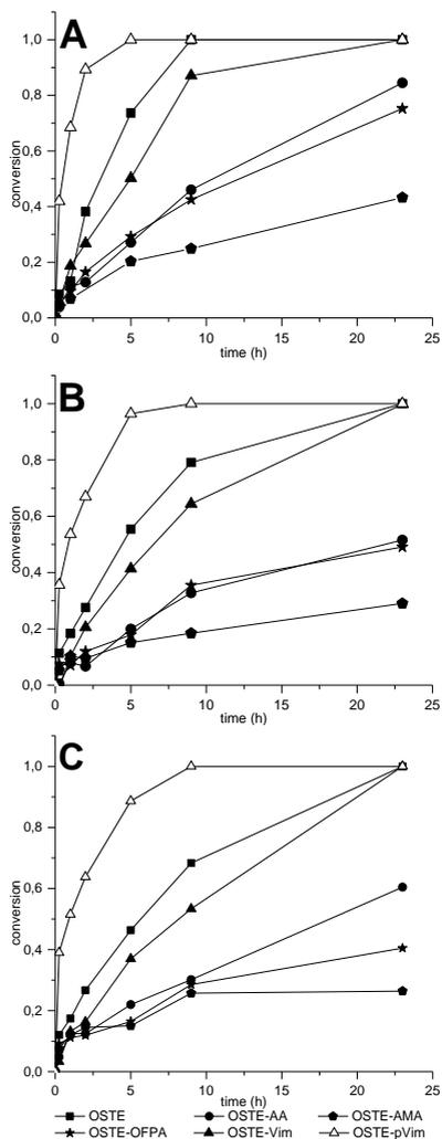
**Figure 2.** Time course of fractional pNPG conversion catalyzed by  $\beta$ -glucosidase immobilized on pristine (OSTE) and functionalized OSTE particles OSTE-AA, OSTE-AMA, OSTE-OFPA, OSTE-Vim and OSTE-pVim in reaction solution, containing (A) 5 vol% , (B) 2 vol% and (C) 1 vol% 1-propanol
