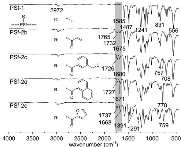
**Figure 7-3** IR spectra of initial PSf membrane (PSf-1) and activated PSf membranes PSf-2 with various acid chlorides, PSf-2b: methacryloyl chloride, PSf-2c: 3-(chloromethyl)benzoyl chloride, PSf-2d: 1-naphthoyl chloride, PSf-2e: 2-furoyl chloride
