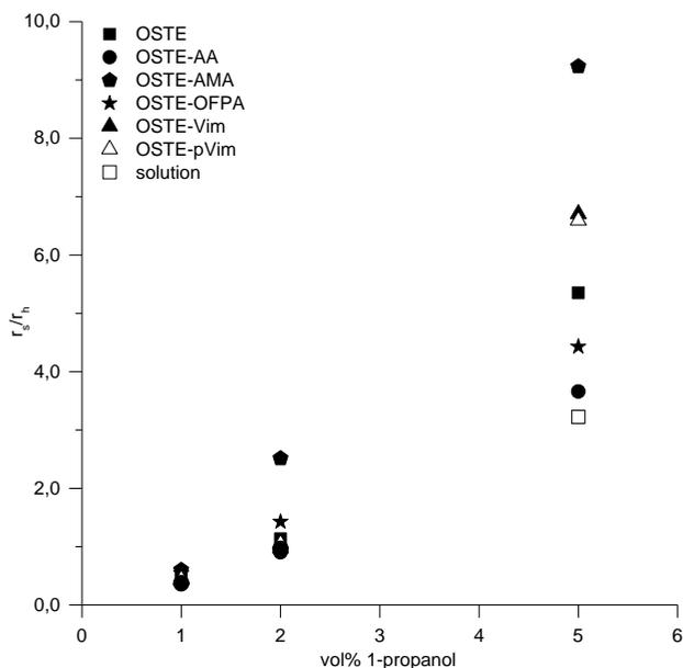
**Figure 5-5** Selectivity ( $r_s/r_h$ ) between trans-glycosylation (s) and hydrolysis (h) of pNPG catalyzed by  $\beta$ -glucosidase immobilized on pristine (OSTE) and functionalized OSTE particles OSTE-AA, OSTE-AMA, OSTE-OFPA, OSTE-Vim and OSTE-pVim at different 1-propanol contents
