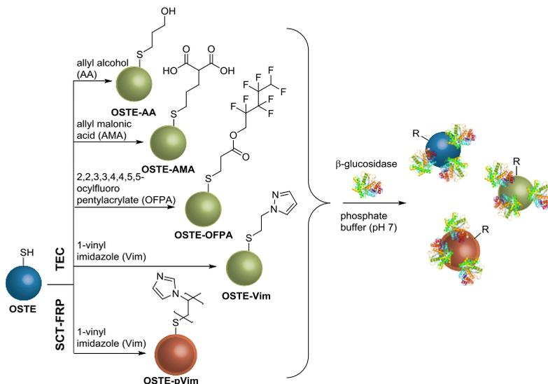
**Scheme 1.** Surface functionalization of OSTE particles via thiol-ene chemistry (TEC) using Vim, AA, AMA, and OFPA to introduce a functional monolayer; and via surface chain transfer free radical polymerization (SCT-FRP) using Vim to graft the surface with a dense polymer layer (pVim) followed by immobilization of  $\beta$ -glucosidase on pristine and functional OSTE particles
