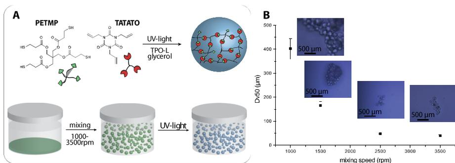
**Figure 1.** A) Preparation of OSTe microparticles via suspension in a speedmixer followed by subsequent photochemical cross-linking of PETMP and TATATO. B) Particle size (Dv50) as a function of mixing speed with optical microscopy images (50 x magnification) of the OSTe particles.
