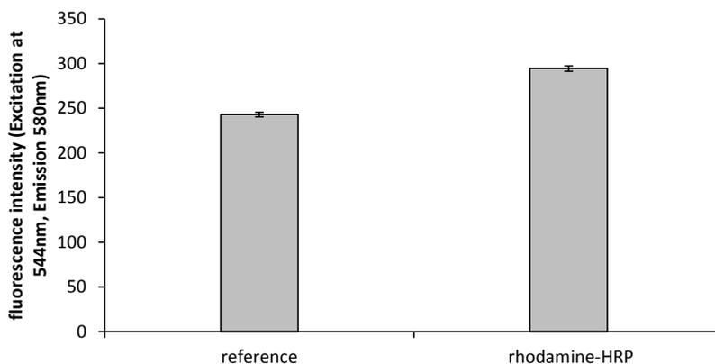
**Figure 3** Fluorescence intensity measurements of a plane thiol-ene surface compared to a thiol-ene surface activated with epoxides (with allyl glycidyl ether) and covalently immobilized rhodamine labeled horseradish peroxidase (HRP)
