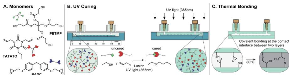
**Figure 6-2** Schematic representation of the preparation of OSTE+ microchips with subsequent surface modification. A) Monomers for OSTE+ preparation tetra functional thiol PETMP, trifunctional allyl TATATO and bifunctional BADGE. B) First UV curing of the OSTE+ mixture via thiol-ene reaction followed by C) a second curing that seals the system “leakage free”
