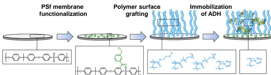
**Figure 7-1** Schematic representation of surface functionalization of PSf membranes by a two-step process including lithiation and acylation, followed by polymer grafting, which allowed the immobilization of ADH
