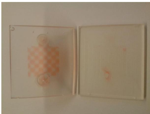
**Figure 2** Photograph of disassembled microreactor after thiol-ene surface reaction with allyl disperse red, left: functionalized top part of microreactor, right: not functionalized bottom part of microreactor
