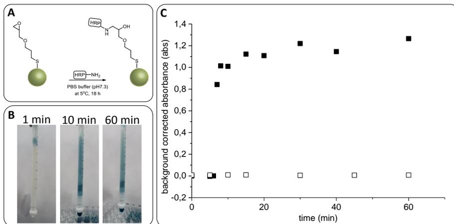
**Figure 4-5** A) Immobilization of HRP on OSTE-AGE particles. B) Photographs of plug-flow reactor at 1 min, 10 min and 60 min of reaction time using a flow of 0.2 ml min<sup>-1</sup> during a ABTS/H<sub>2</sub>O<sub>2</sub> activity measurement of immobilized HRP on OSTE-AGE particles. C) Enzyme activity as background corrected absorbance at 412 nm over time of OSTE-AGE particles with immobilized enzyme (full squares) and a reference (without enzyme -empty squares)
