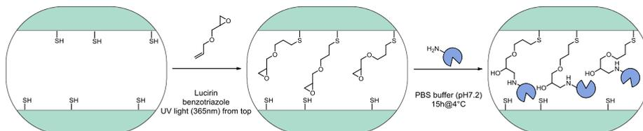
**Figure 6-4** Microchip functionalization of remaining surface thiol groups using allyl glycidyl ether via UV initiated thiol-ene reaction and subsequent covalent HRP immobilization with introduced epoxide groups on the microreactor surface
