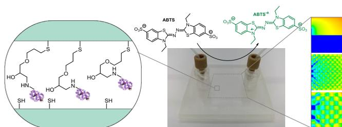
**Figure 6-1** Illustration of fabricated microreactors including the area selective immobilization of horseradish peroxidase (HRP) and subsequent reactor performance tests using ABTS as a colorimetric assay
