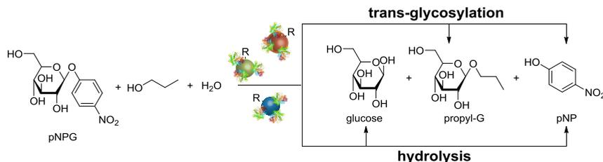
**Scheme 5-2** Enzymatic conversion of p-nitrophenyl  $\beta$ -D-glucopyranoside (pNPG) catalyzed by  $\beta$ -glucosidase immobilized on pristine and functional OSTE particles, in order to determine the biocatalytic activity and selectivity between trans-glycosylation with 1-propanol forming propyl-glucoside (propyl-G) and p-nitrophenol (pNP) as products and hydrolysis with water forming glucose and pNP as products
