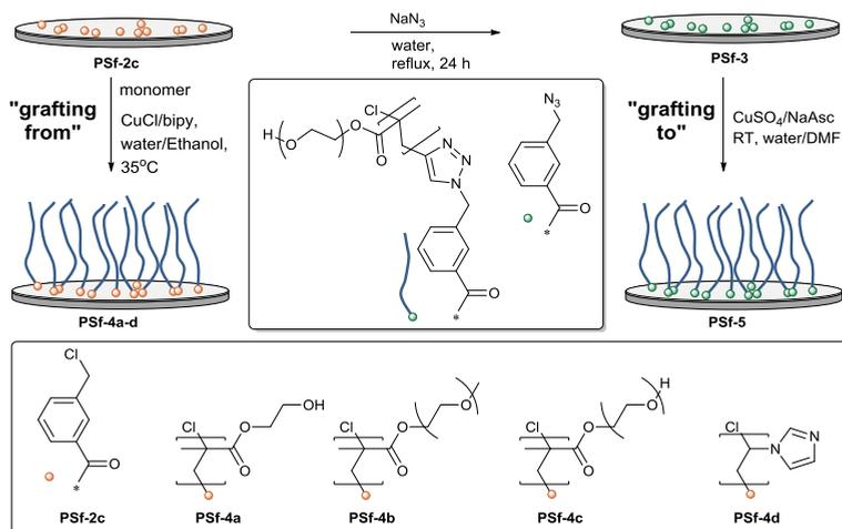
**Scheme 7-2** Two surface grafting approaches: “Grafting from” by SI-ATRP of the chloride functionalized PSf membranes (PSf-2c) to provide PSf-4a-d; azidation of PSf-2c, leading to PSf-3, followed by “Grafting to” through CuAAC with alkyne functionalized polyPEGMA, resulting in PSf-5
