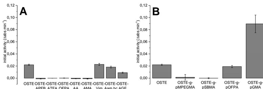
**Figure 3-5** Initial enzyme activity of Rho-HRP immobilized on virgin (OSTE) and functionalized surfaces via TEC (A) with various ene compounds and SCT FRP (B) with various acrylate and methacrylate based polymers
