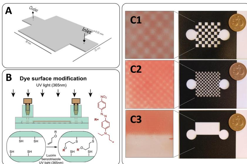
**Figure 6-3** A) Microreactor geometry, B) Microreactor surface modification via TEC using allyl disperse red, C1-3) Images of surface functionalized microchips using allyl disperse red and different stencil masks: C1 – coarse checkerboard, C2 – fine checkerboard, C3 - half reacted surface
