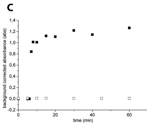
*Figure 3.* A) Immobilization of HRP on OSTE-AGE particles. B) Photographs of plug-flow reactor at 1 min, 10 min and 60 min of reaction time using a flow of  $0.2 \text{ ml min}^{-1}$  during a ABTS/ $\text{H}_2\text{O}_2$  activity measurement of immobilized HRP on OSTE-AGE particles. C) Enzyme activity as background corrected absorbance at 412 nm over time of OSTE-AGE particles with immobilized enzyme (full squares) and a reference (without enzyme -empty squares)
