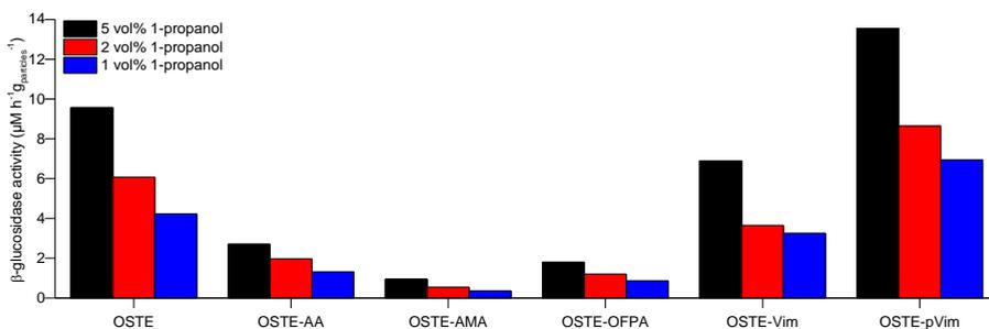
**Figure 5-3** Activity (combined initial reaction rates of trans-glycosylation and hydrolysis) of  $\beta$ -glucosidase immobilized on pristine (OSTE) and functional OSTE particles in solutions with different 1-propanol contents, such as 5, 2 and 1 vol%
