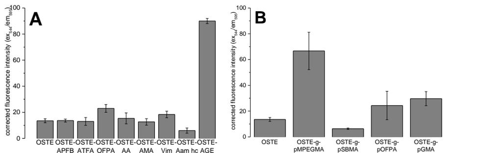
**Figure 3-4** Reference corrected fluorescence intensity of virgin (OSTE) and functionalized surfaces via TEC (A) and SCT-FRP (B) after immobilization of rhodamine labeled horseradish peroxidase (Rho-HRP), excitation at 544 nm and emission at 595 nm
