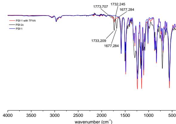
**Figure S1** IR spectra of virgin membrane (PSf-1), reacted membrane with trifluoroacetic anhydride (TFAA, PSf-1 with TFAA) and as comparison the IR spectrum of PSf-2c (membrane reacted with acid chloride after lithiation)
