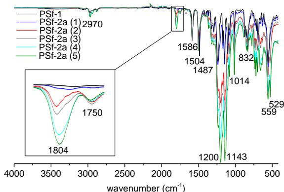
**Figure 7-2** IR spectra of PSf membrane (PSf-1) and activated PSf membranes PSf-2a (1)-(5) with pentadecafluorooctanoyl chloride with increasing n-BuLi concentration from 1.16  $\text{mmol}_{\text{n-BuLi}} \text{g}_{\text{membrane}}^{-1}$  (PSf-2a (1)) until 39.8  $\text{mmol}_{\text{n-BuLi}} \text{g}_{\text{membrane}}^{-1}$  (PSf-2a (5)), magnification in the wavelength range of 1720 to 1860  $\text{cm}^{-1}$
