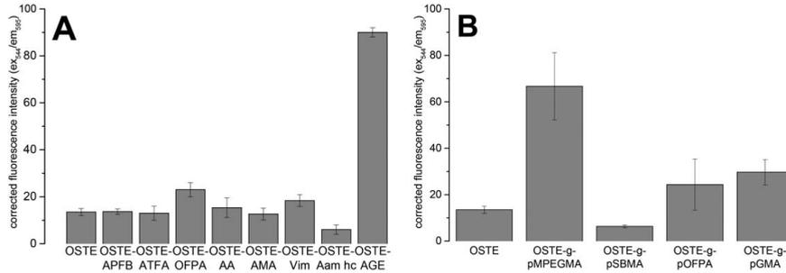
**Figure 3.** Reference corrected fluorescence intensity of virgin (OSTE) and functionalized surfaces via TEC (A) and SCT FRP (B) after immobilization of rhodamine labeled horseradish peroxidase (Rho-HRP), excitation at 544 nm and emission at 595 nm, standard deviations are based on three experimental replicates ( $n = 3$ ).
