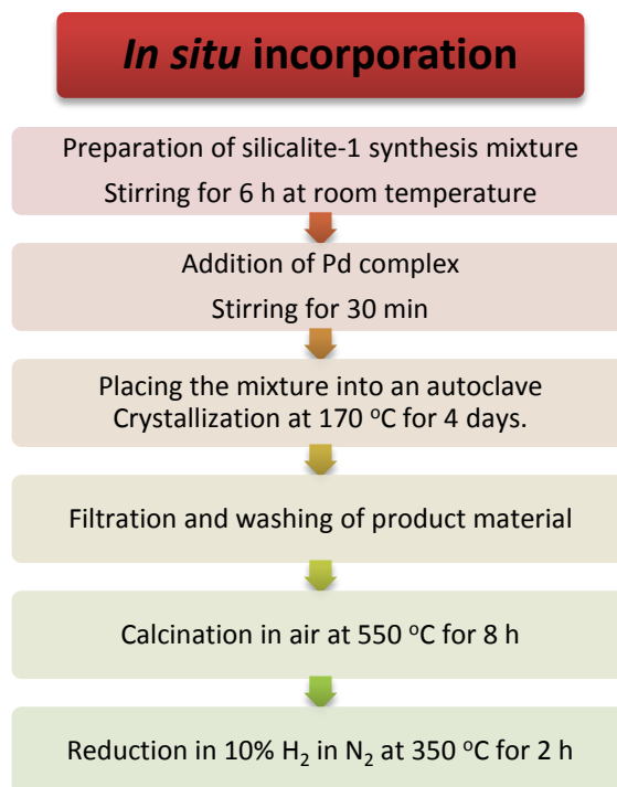
Figure 1.2. Schematic representation of the in situ incorporation methodology used in this study for the synthesis of metal nanoparticles encapsulated inside silicalite-1.
