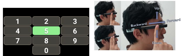
(a) Demonstration of gTapper. (b) The top left figure, bottom left figure, and right figure show one-finger operations, two-finger operations, and swiping directions, respectively.
