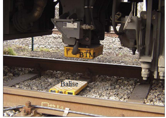
Fig. 2. Balise is mounted between the tracks, and a Balise Transmission Module (BTM) is mounted on the train. They cooperate to fulfill the track–train telegram transmission [16].
