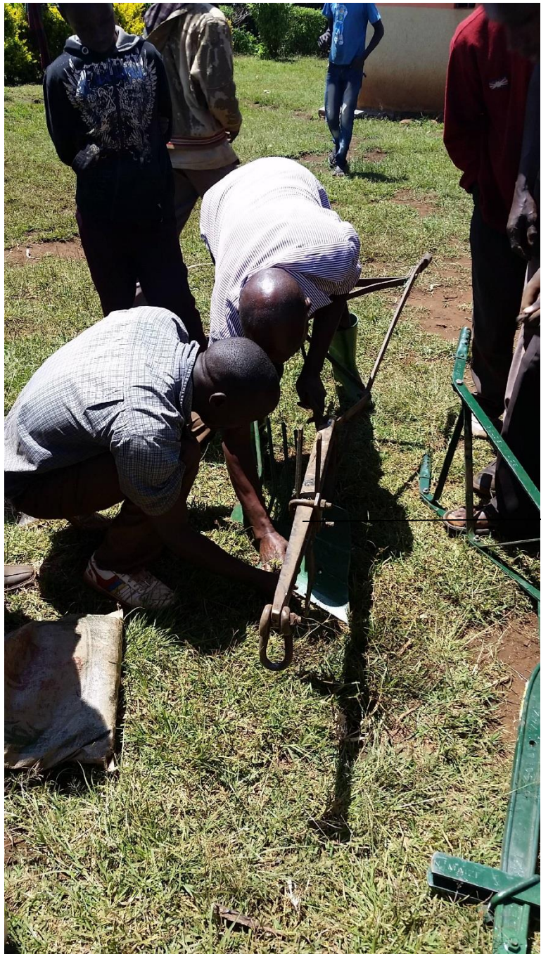
Figure 5: Innovative farmer transferring forked/pronged attachment onto Sebei frame which has a much shorter beam and share than ordinary plough frame (brown frame) with pronged end (green) replacing the mouldboard
