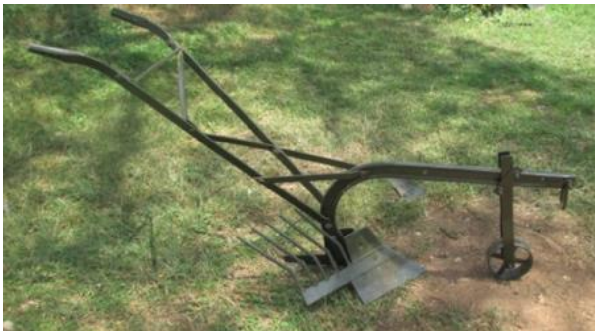
Figure 1: NARO ox-drawn potato lifter, with a mouldboard replaced by pronged fork
