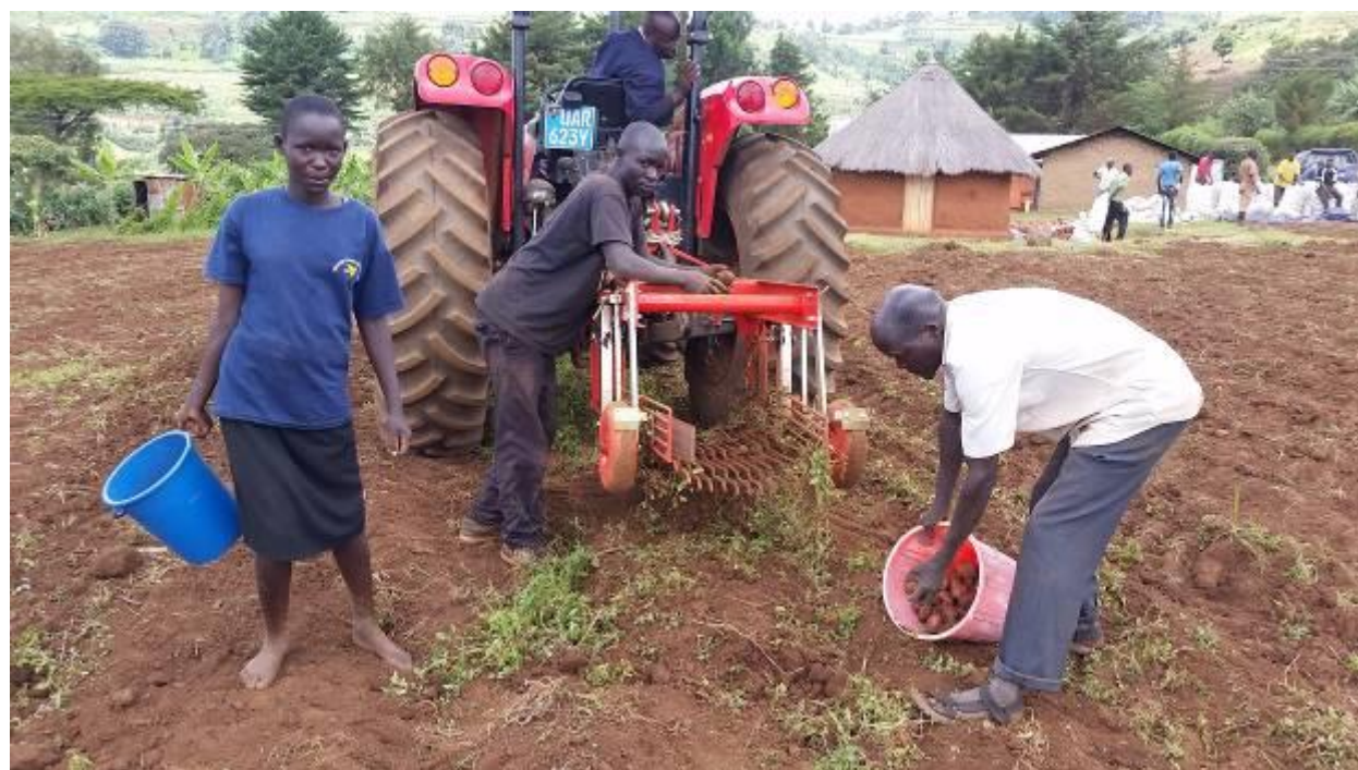
Figure 7: Potato lifter mounted on 3 point of a tractor in field after harvesting
