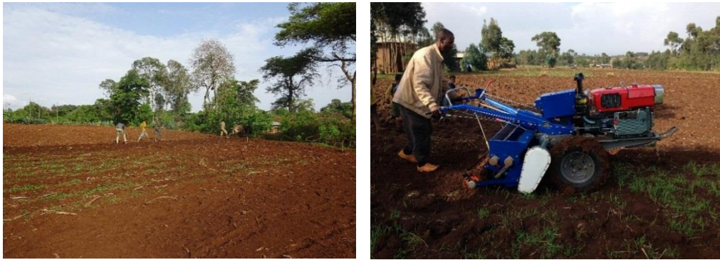
Photo 4: Planting using the conventional animal drawn maresha system (left picture) and service provider planting teff using a 2 WT drawn planter (right picture) in Ethiopia
