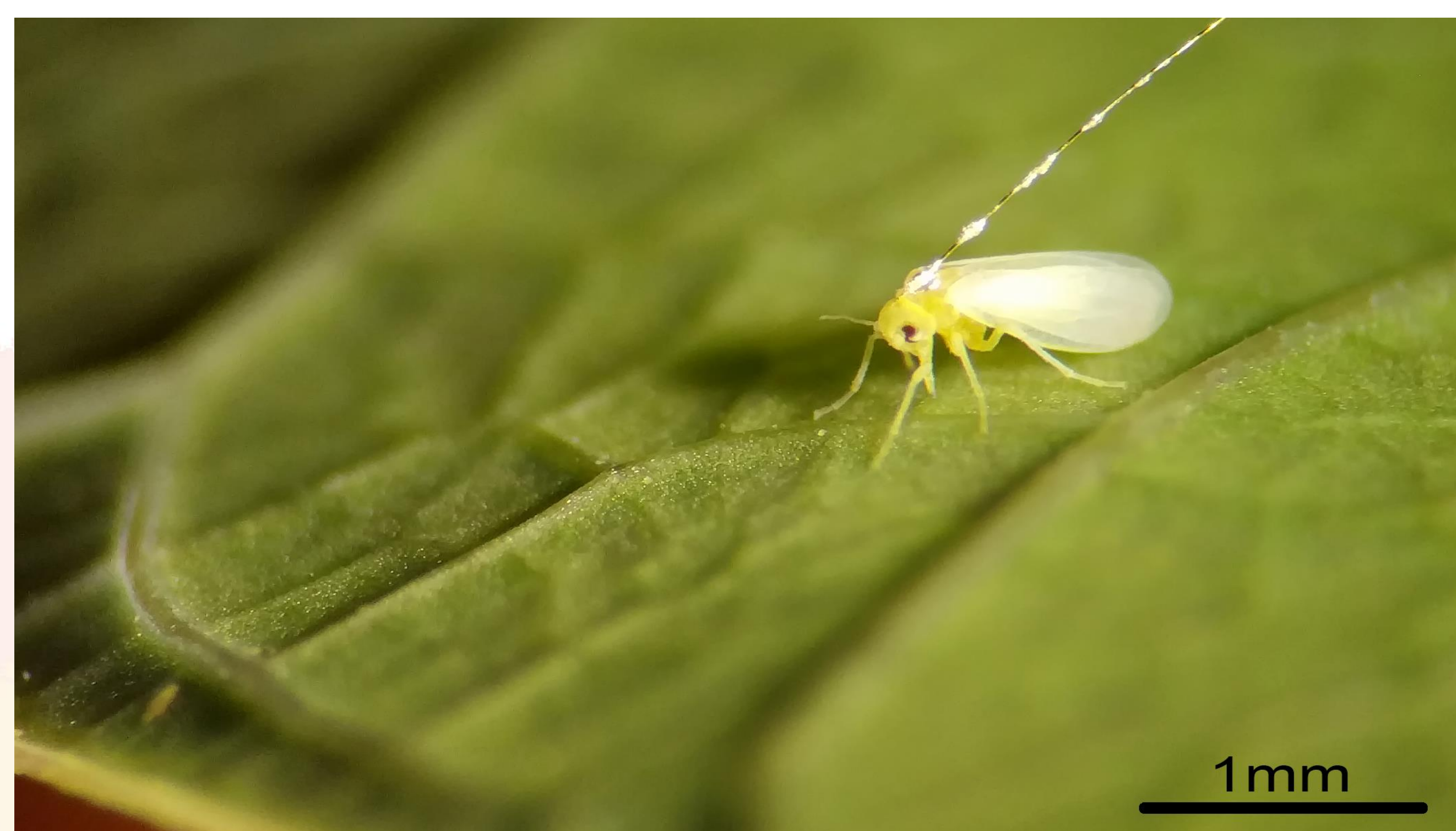
Fig. 2: Whitefly attached to a 12.5µm gold wire using water-based silver glue.
