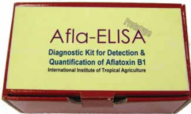
Prototype Afla-ELISA kit—a quantitative serological assay for the estimation of total aflatoxins in maize and other commodities, using 96-well microtiter plates. Up to 20 samples can be tested in each 96-well plate at a cost of US$4 per sample. Source: L Kumar.
