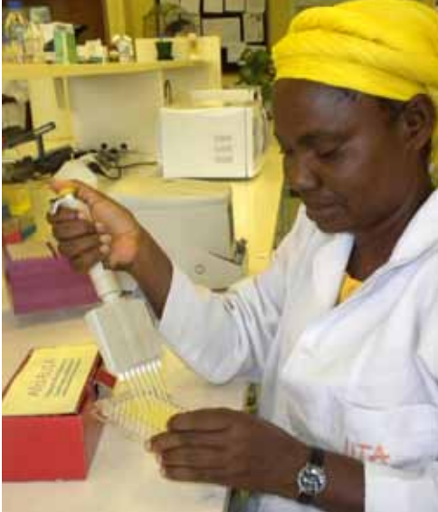
Aflatoxin testing using Afla-ELISA. Source: L. Kumar
