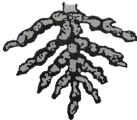
5. Severe galling damage
