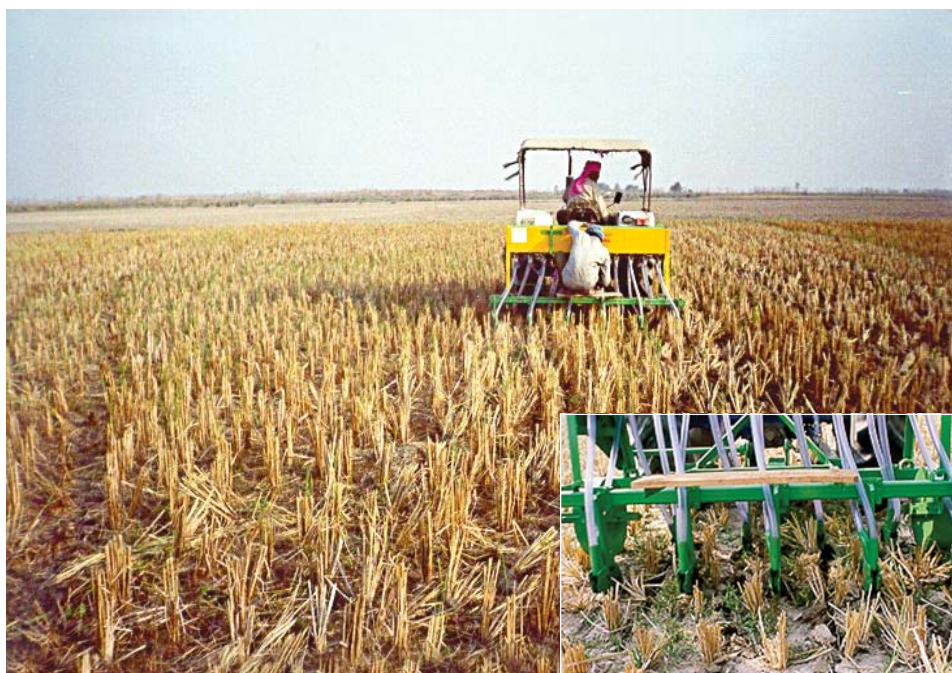
Fig. 2. Zero-till drill sowing wheat in the untilled rice fields. Inset: A close-up of the seeder
