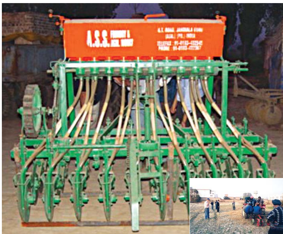
Fig. 1. Newly developed zero-till drill which is capable of seeding into loose residues avoiding burning residues considerably (Inset: Manufacturers, scientists and farmers worked together in developing and testing the prototype of new zero-till drill)
