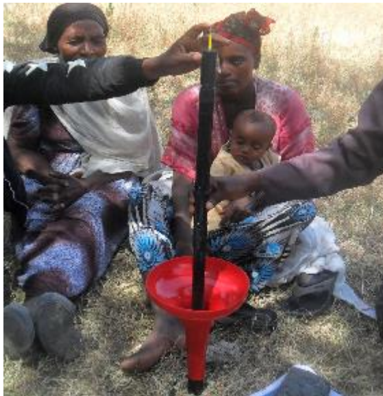
Figure 1. A Full Stop WFD. The funnel part is buried in the soil with the black tube protruding above the soil surface. When a wetting front reaches the detector, an indicator pops up.
