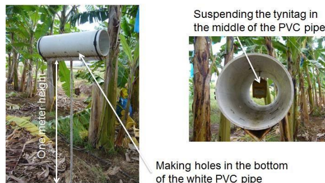
Figure 1. On-field thermal data logger installation
