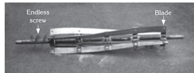
Figure 23-5. A mill shaft.
