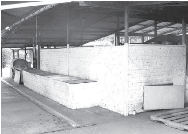
Figure 22-14. CLAYUCA's artificial fixed-bed dryer at CIAT, Palmira.
