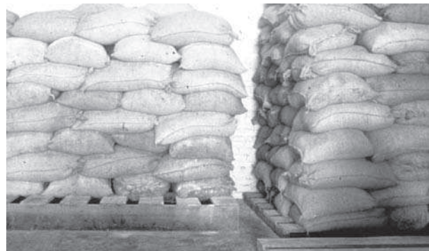
Figure 21-12. In the storeroom, sacks of dried cassava chips should be stacked on pallets or wooden platforms.
