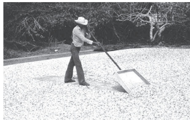
Figure 21-8. Dried cassava chips are collected by piling them up in the concrete floor, using a wooden shovel.
