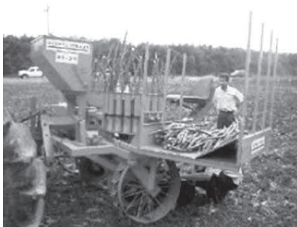
Figure 20-8. Two-furrow cassava planter, model PC-20.
