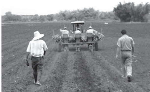
Figure 20-9. Three-furrow cassava planter, model PMT-3.
