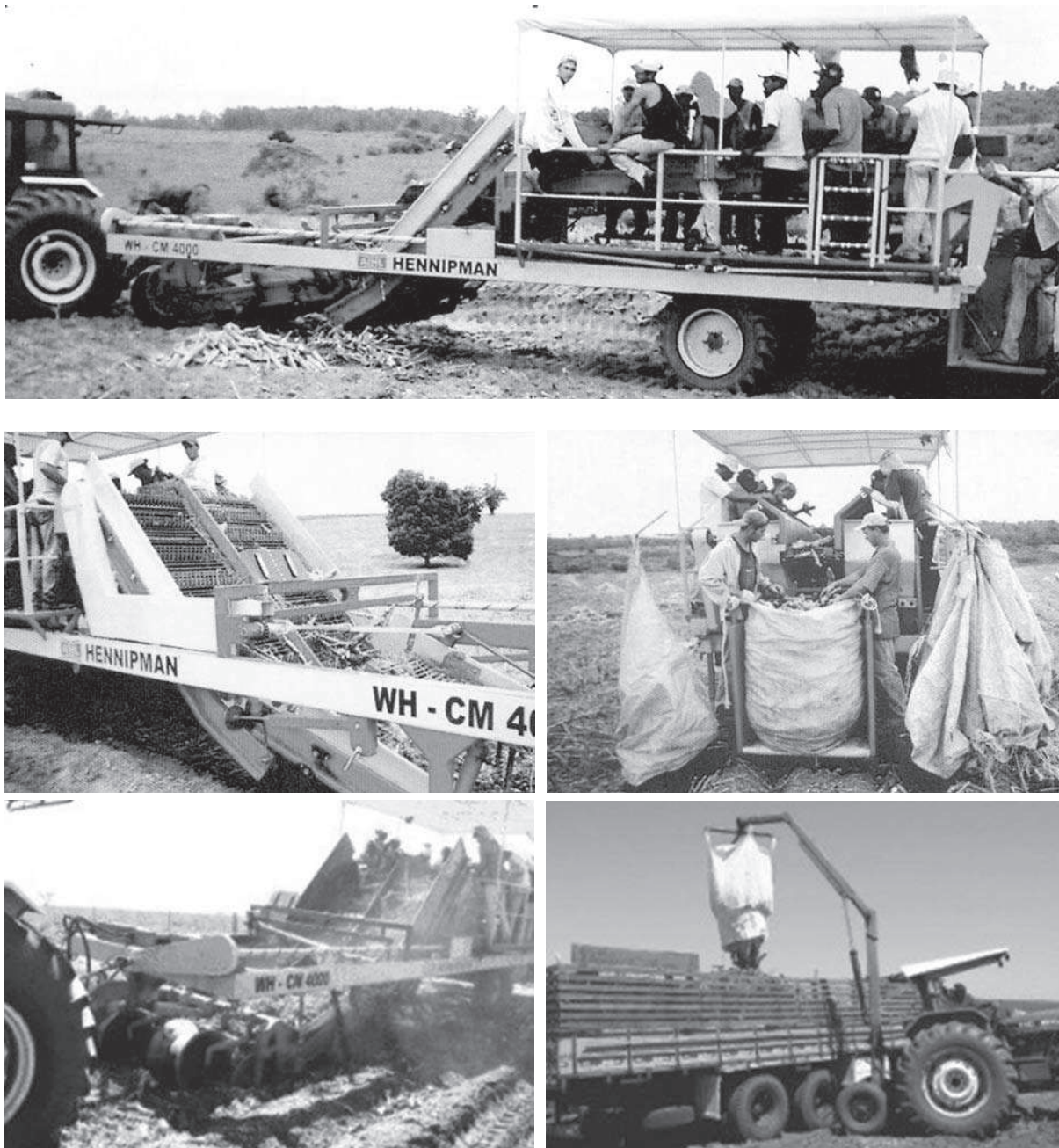
Figure 20-22. Prototype of mechanical harvester, model WH-CM 4000. Also shown are the use of the big-bag sack (central right) and the winch in operation (bottom right).
