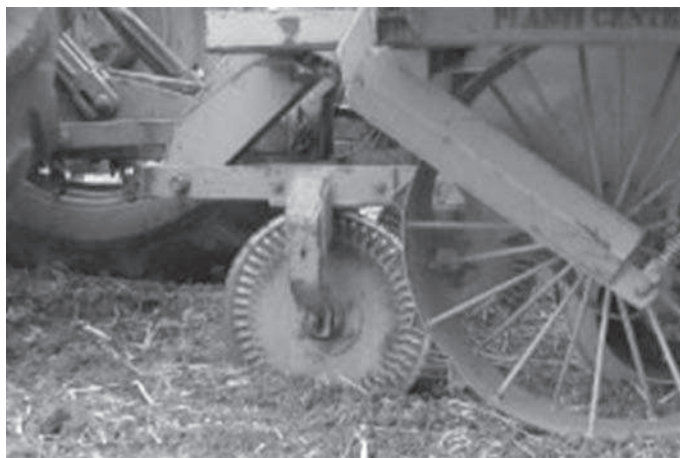
Figure 20-14. Two angles of the direct-planting device in the 2-furrow cassava planter, Planti Center model PC-20.
