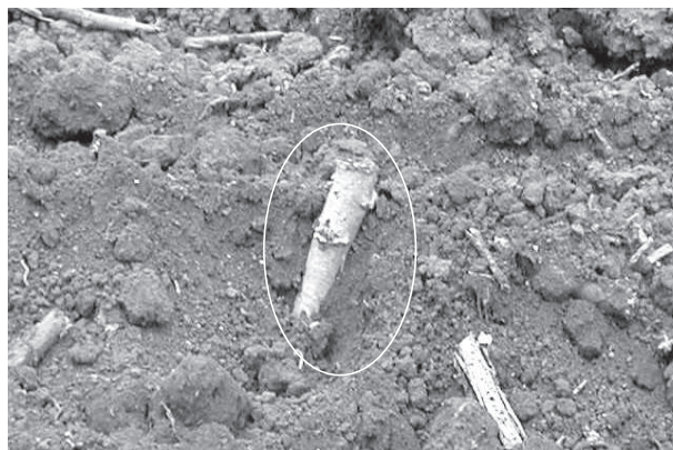
Figure 20-4. Stake planted on a slant.
