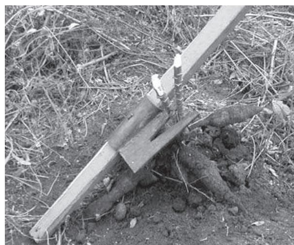
Figure 20-17. Puller used by Thai farmers to harvest cassava.
