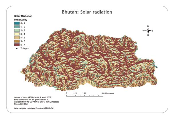
Figure 11: Solar radiation map in kwh/m<sup>2</sup>/day
