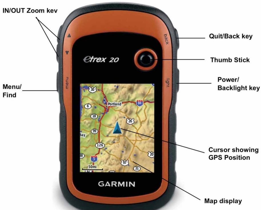
Figure 4: Garmin Etrex 20 GPS device and main uses of the buttons.
