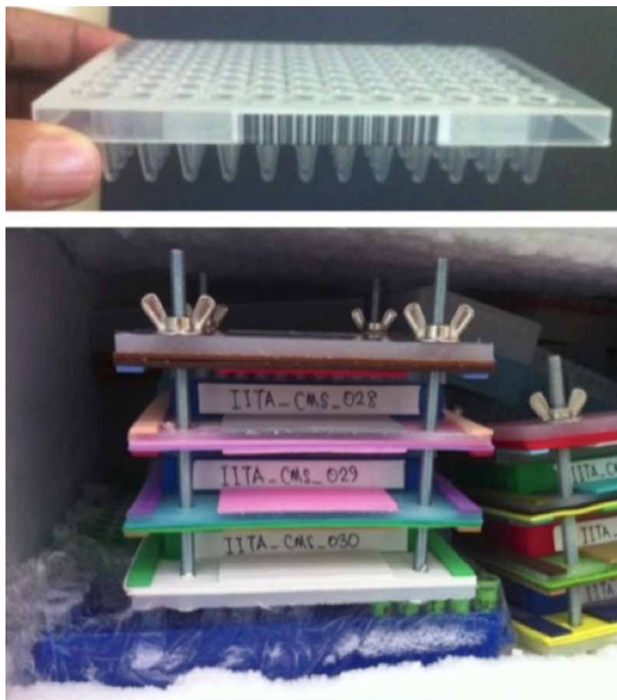
Figure 8: Samples arranged in a stack (with barcode labels pasted on each plate) in addition to plate ID information.
