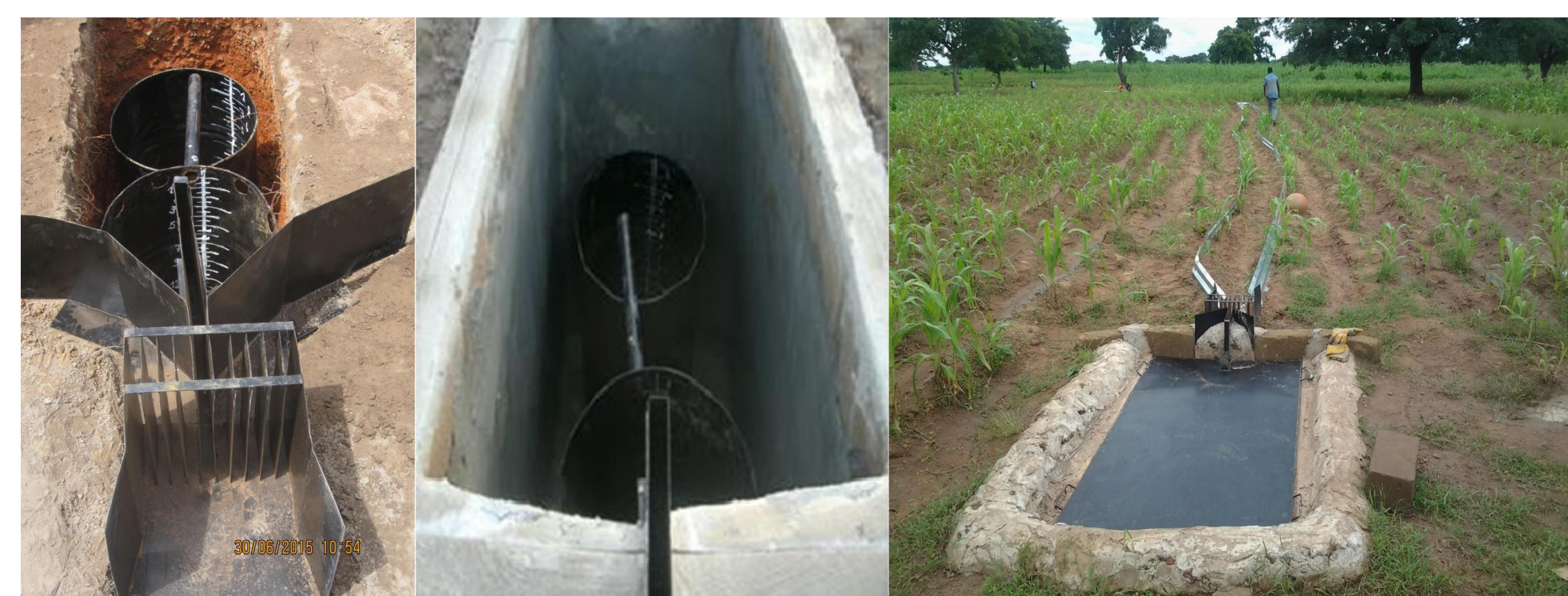
Figure 2. Layout of runoff and erosion measurement in Flola technology park, southern Mali
