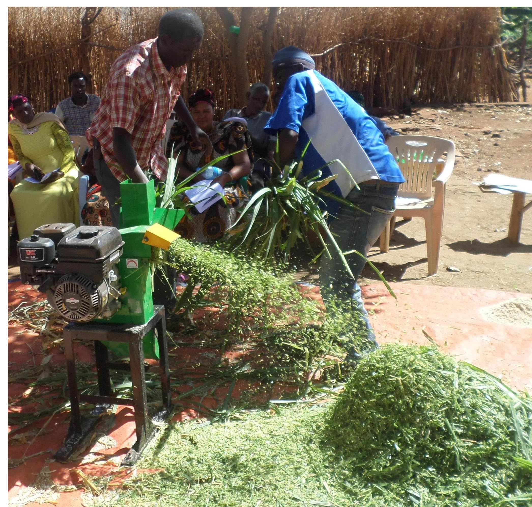
Figure 2. Demonstration of grinding different ingredients for feed rationing with a chopper machine.
