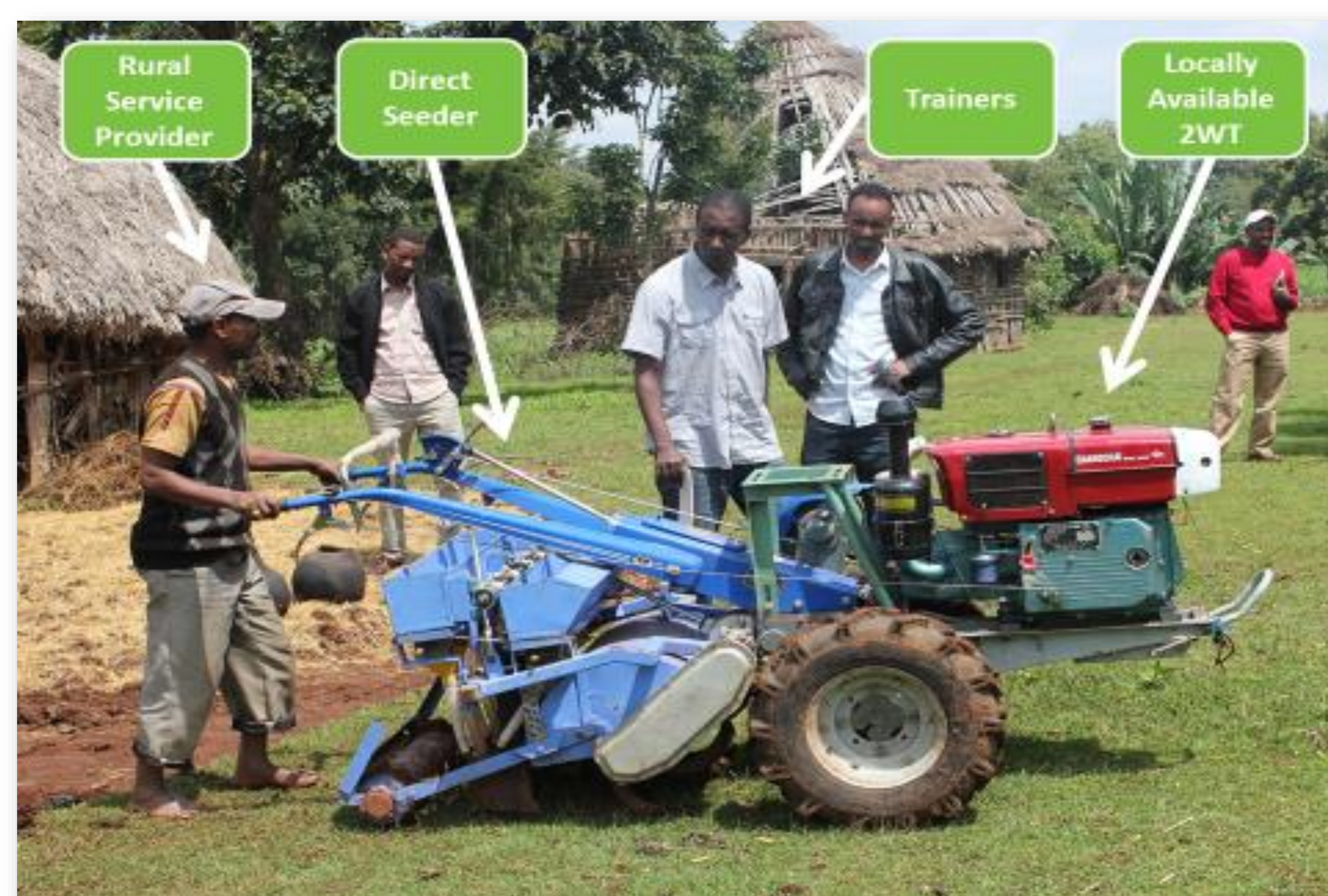
Our approach to appropriate mechanization summarized in one picture: a direct seeder powered by a locally available two-wheel tractor (2WT) operated by a rural service provider receiving continuous training.
