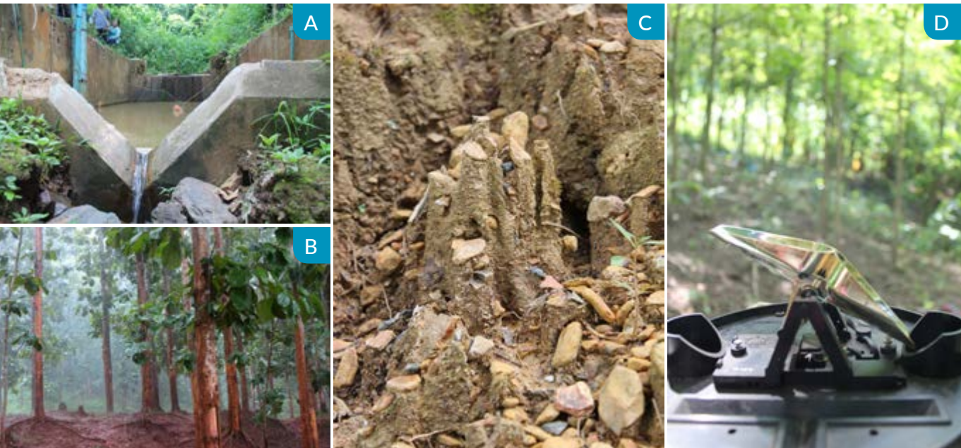
Photo 3.1 The research site in Laos: Houay Pano catchment, part of the ‘Multi-Scale Environmental Change’ (MSEC) network. A: Stream water level measured within a V-notch weir by a water level recorder equipped with a data logger. B: Teak plantation in the rain. Root exposure illustrates ongoing erosion. C: Small fairy chimneys on steep soil in a teak plantation, revealing intense erosion rates. D: Tipping bucket rain-gauge used to monitor rainfall. Photo credits: IWMI/Guillaume Lacombe
