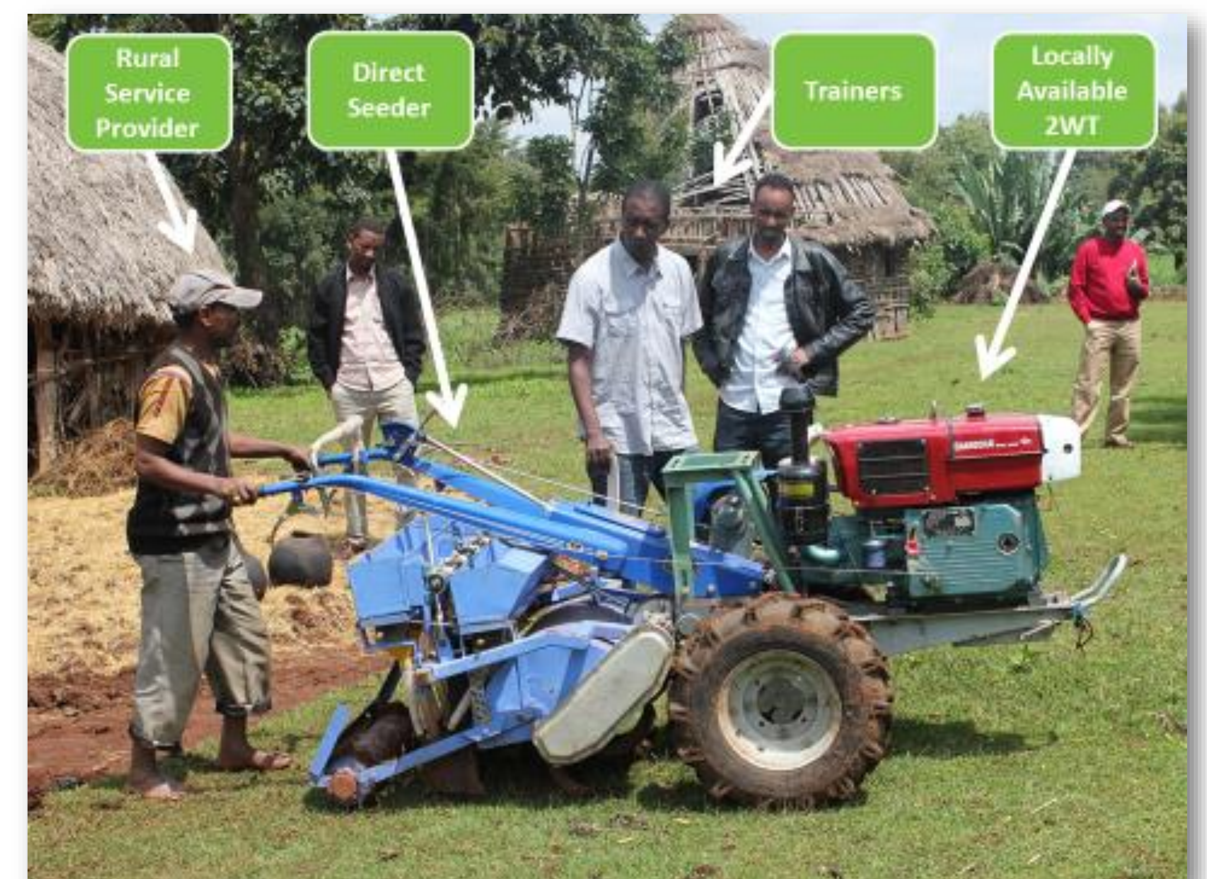
Our approach to appropriate mechanization summarized in one picture: a direct seeder powered by a locally available two-wheel tractor (2WT) operated by a rural service provider receiving continuous training.
