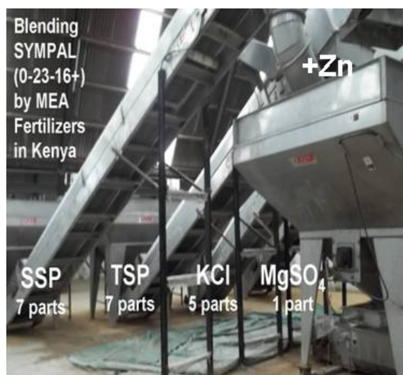
Figure 4.4: Fertilizer blending of Sympal at the MEA Ltd. factory in Nakuru, Kenya.
