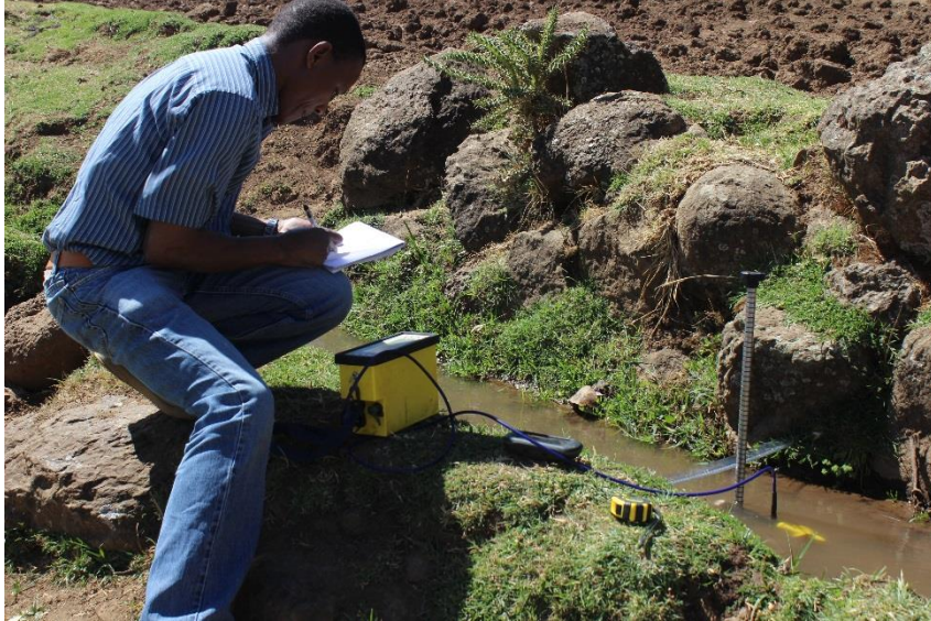
Photo 3: Taking flow velocity readings along Group 1 Main Canal reach
