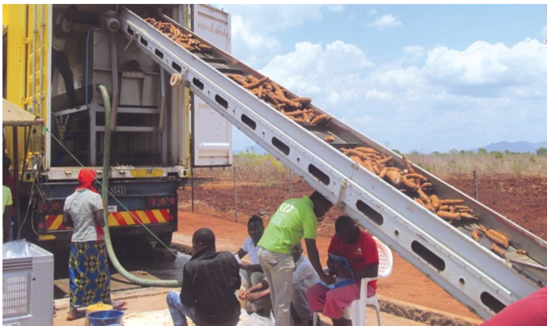
Workers deposit fresh cassava on the conveyer belt—the process continues with the washing & peeling phase
