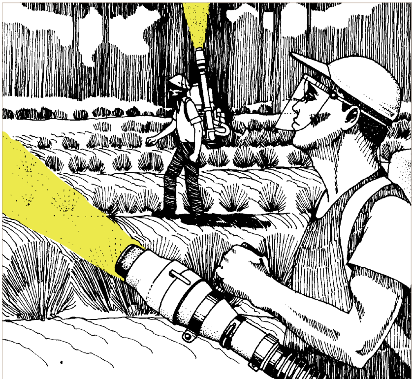
Figure 37. Backpack mist blower fitted with AU8000 spray head (after Micronair).
