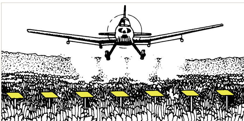
Figure 27. – Arrangement of droplet collectors aircraft spraying water-based formulation (after Ciba-Geigy). The papers are placed horizontally under the flying aircraft.
