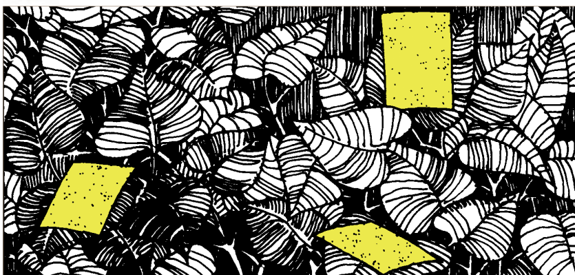
Figure 26. Sensitive papers pinned directly within the canopy at different heights of a shrub like plant (after Ciba-Geigy).
