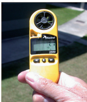
Figure 19. Digital display anemometer. It displays the mean wind speed calculated over 30 consecutive seconds.
