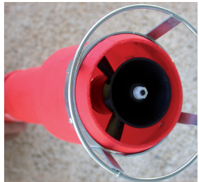
Figure 12. Centrifugal device mounted in the air pipe of a mist blower knapsack sprayer (Micron Sprayers).
