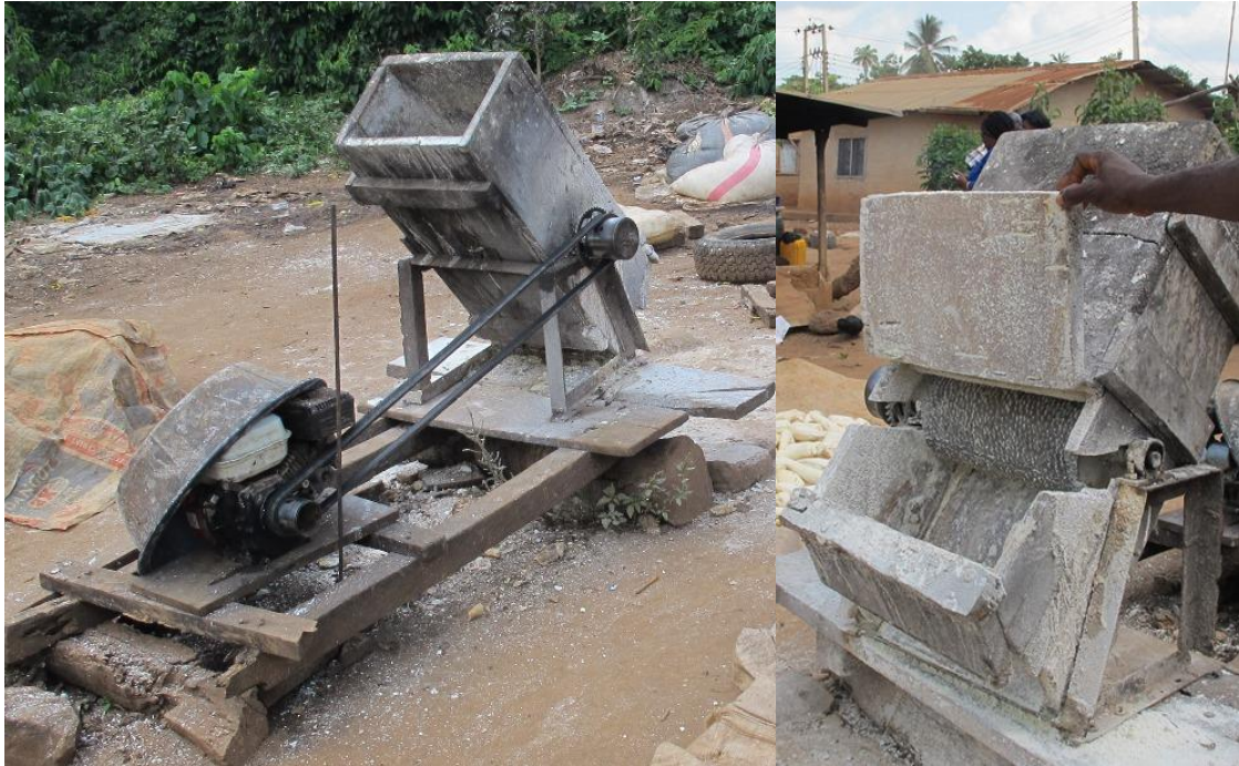
Motorized cassava graters are common labor-saving devices in Nigerian villages
