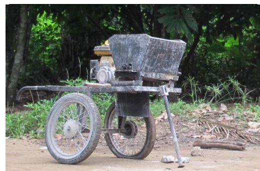
A motorized grater on wheels can be taken from one farm to the next
