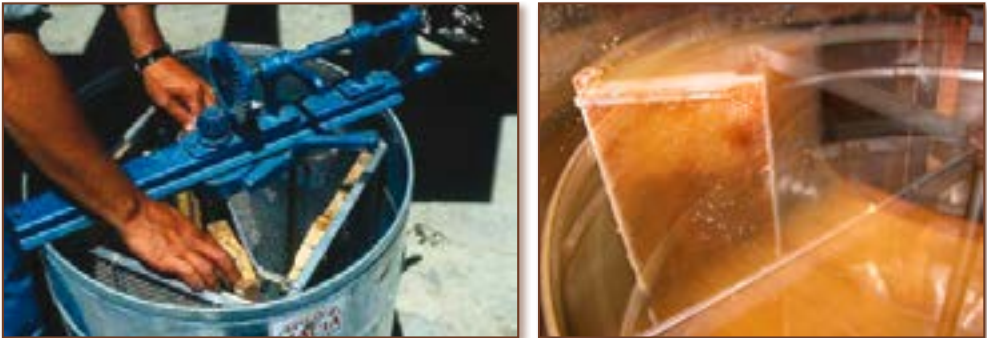
Fig.3.5.4. a) Manual honey extractor (From Krell, 1996), b) Extractor in motion (From Ben pcc)
