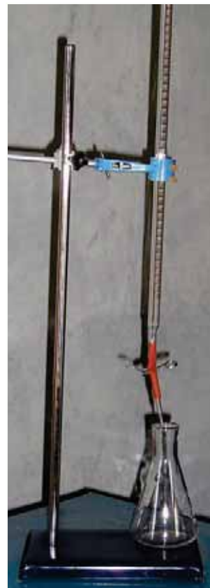
Fig. 5.2 Equipment for measuring acidity (Photo: Peter Fellows)
