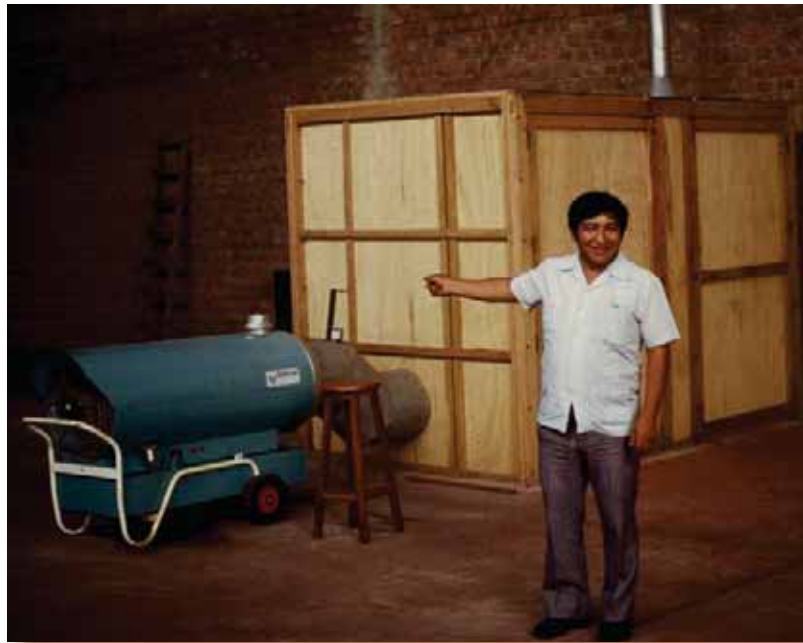
Fig. 3.8 A batch tray dryer (Photo: Barrie Axtell)
