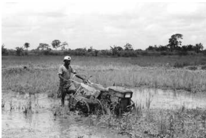
Figure 6: Use of power-tiller for puddling in irrigated rice, southern Togo
