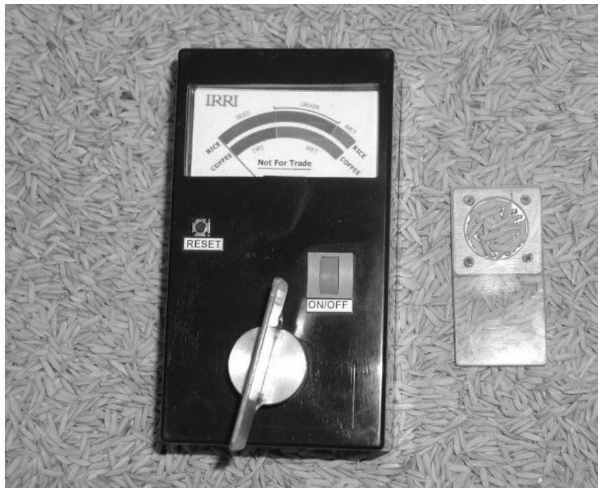
Figure 25: Electronic meter to measure the moisture content of seeds. The operation of the meter is described below.
