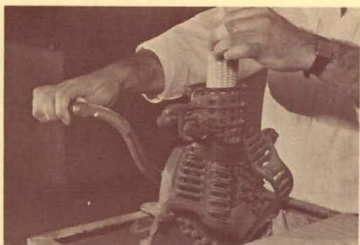
FIGURE 6. Crank hand sheller. Simple to construct and clean; used for shelling maize.
