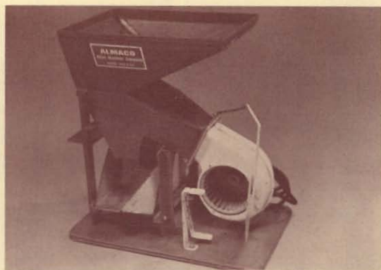
FIGURE 9. Air blast blower (normally used in laboratory for research experiments). Similar to that shown in Figure 8, but motor-driven and constructed from metal. Very appropriate for small amounts of seed. It can be easily adapted to have a constant flow of air.
