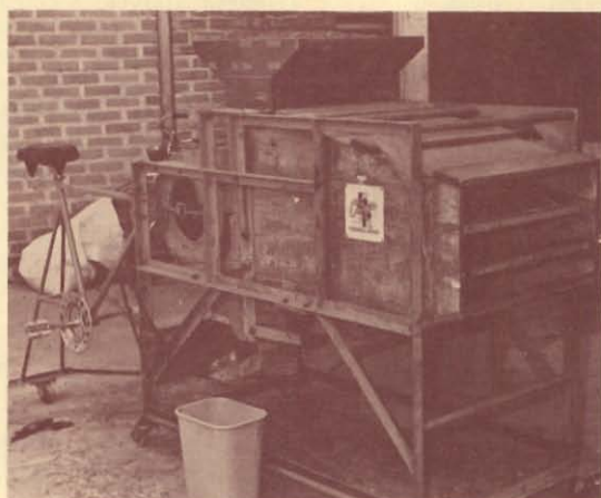
FIGURE 15. Air screen cleaner. Can be activated by pedal or by electric or gasoline engine.
