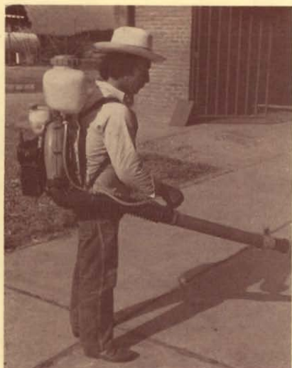
FIGURE 10. Backpack air blower, normally used to apply chemical products in the field. Useful in separating light components (stems, dust, leaves, pods, etc.) after threshing.
