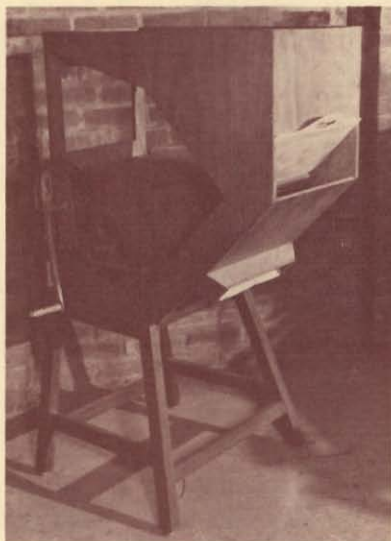
FIGURE 8. Crank blower. Simple machine, easily constructed from wood, very useful for precleaning seed. Can be adapted to be activated by a motor to facilitate operation and increase efficiency.
