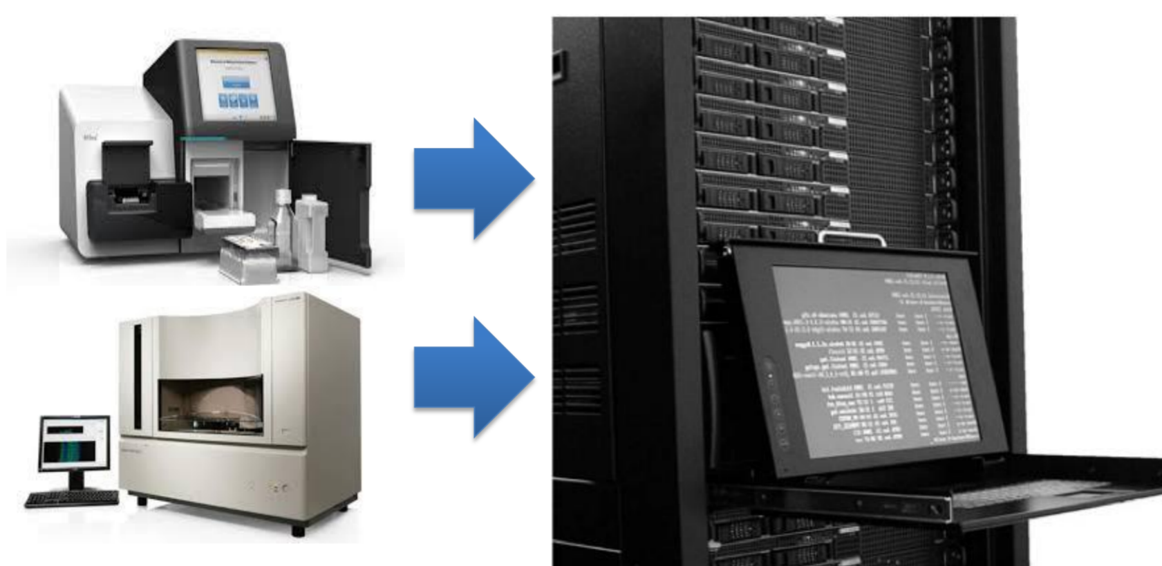
Figure 1. The HPC platform is a 152 CPU Linux cluster, based on AMD 64-bit Opteron technology with a total of 80TB disk storage.
