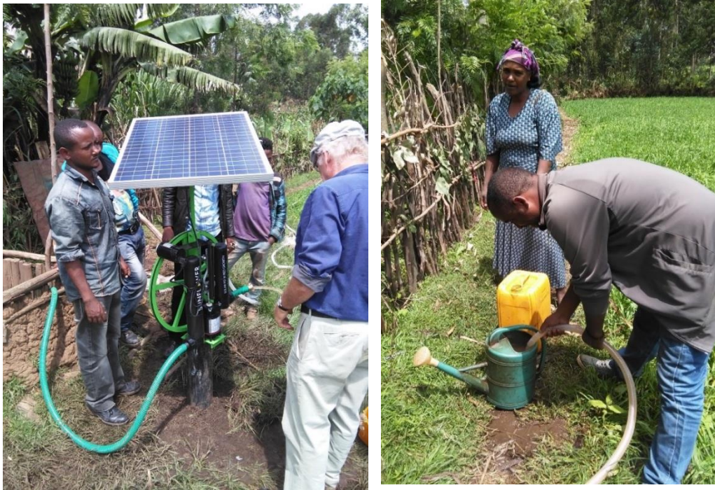
Figure 6 : water pumping from the well using the solar pump and measuring the amount
