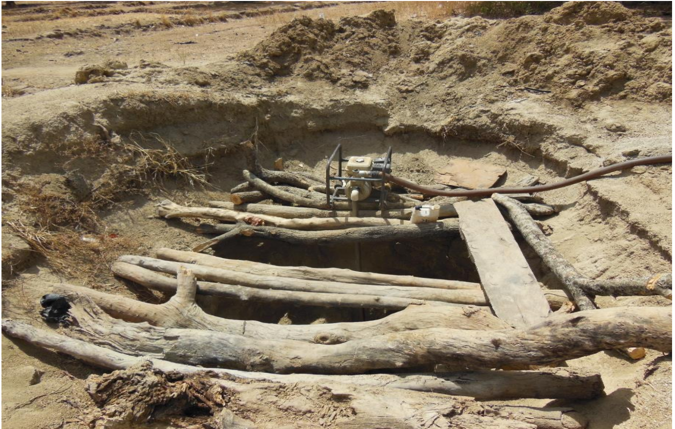
A motorized pump used for small-scale vegetable irrigation in Upper East Ghana. Photo: P. Schmitter
