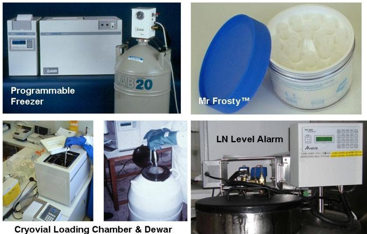
Figure 6. Basic equipment used for the cryopreservation of plant genetic resources: Programmable freezer comprising freezing chamber, computer and pressurized liquid nitrogen coolant; solvent-cooled, passive small-scale freezing unit 'Mr Frosty™', cryovial loading into cooling chamber and small (ca 50 L) storage Dewar, LN level alarm attached to large-capacity (ca 200 L) cryotank.
