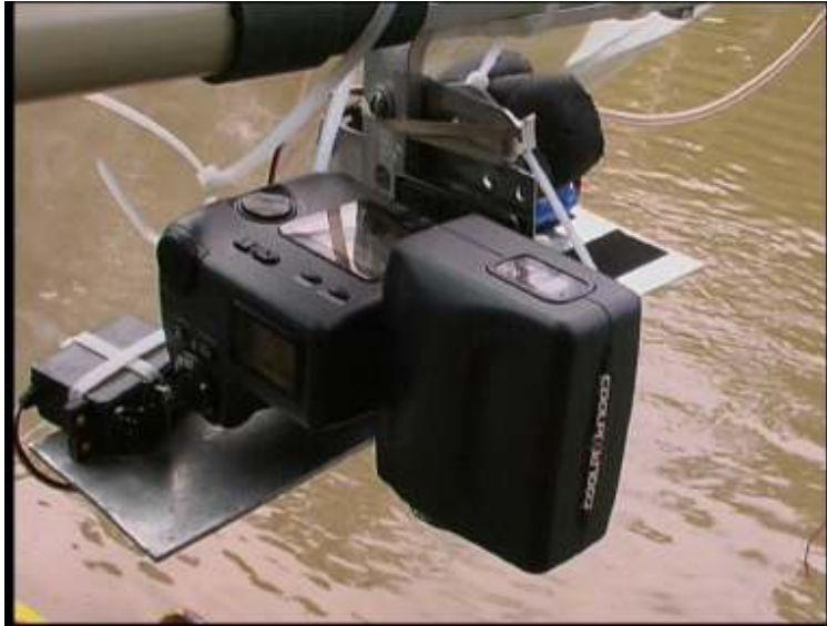
Figure 119 Instrumental setup of tethered balloon photo acquisition
