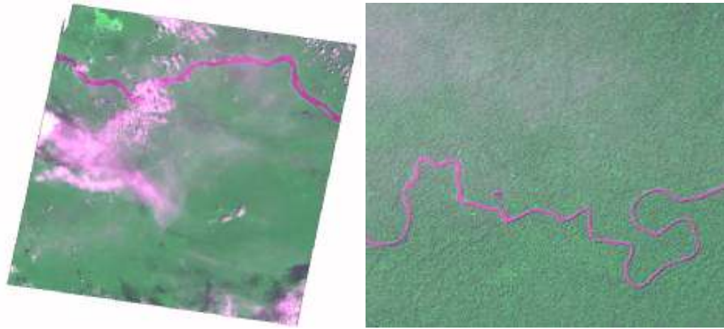
Figure 22 The VNIR ASTER image from 12 th April 2003, used to extract a 15m DEM, displayed using bands 2 (red), 3 (infra-red) and 1 (green). Whole image (left) shows heavy cloud cover in the western and south-eastern sector of the image, but TBS is cloud free (right).
