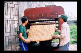
5. Mats are pressed together under high temperature and pressure to form roofing sheets
