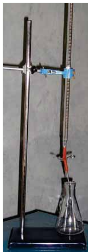
Fig. 5.2 Equipment for measuring acidity (Photo: Peter Fellows)
