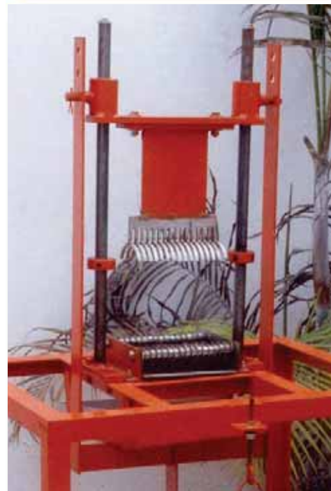
Fig. 3.5 Pineapple corer (above) and slicer (below) (Photo: Barrie Axtell)
