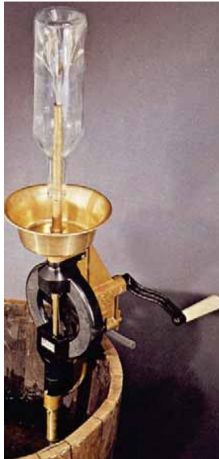
Fig. 3.3 Manual rotary bottle-cleaning brushes (Courtesy of Sanbri Ltd.)
