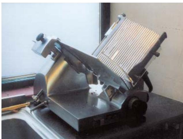
Fig. 4.33 Self-sharpening, adjustable meat slicer
