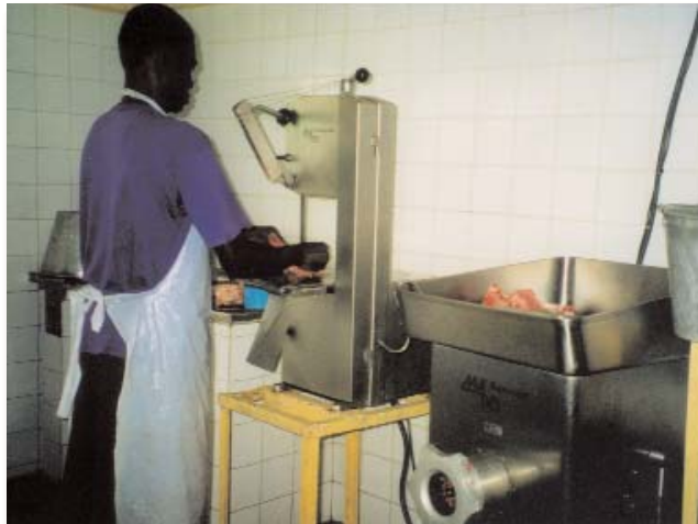
Fig. 4.9 A small band saw (Photo: R. Zulu)
