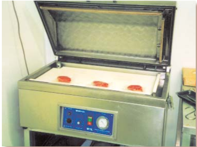
Fig. 4.15 Tabletop vacuum packing machine (Photo: B. Axtell)
