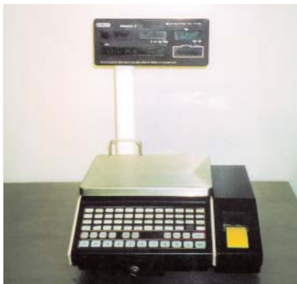
Fig. 4.8 Automatic net weight label printer (Photo: B. Axtell)
