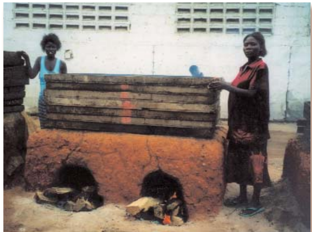
Fig. 5.7 Brick-built smoker with external firebox (Photo: P. Oti-Boateng)
