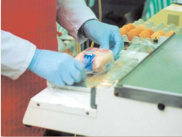
Fig. 4.19 Over-wrapping sausages with shrink film (Photo: B. Axtell)
