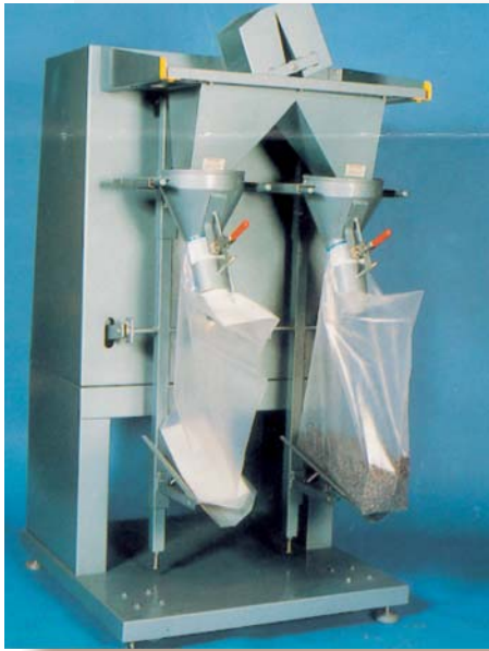
Fig. 3.13 Manual bagging machine for flour (Photo: courtesy of A.T. Sack Fillers-Simplafill Systems Ltd)
